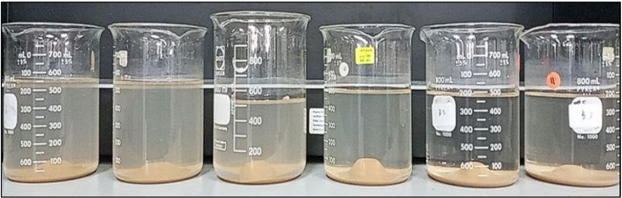
Figure 4. The settling floc after the experiment
